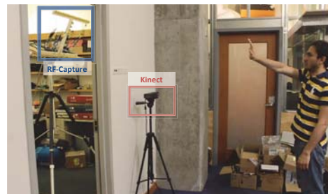
Figure 12—Tracking the Human Hand Through Walls. RF-Capture tracks the subject’s palm through a wall while the Kinect tracks it in line-of-sight.
